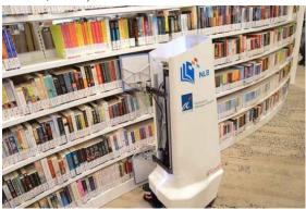
AuRoSS (autonomous robotic shelf scanning system), a robot that can navigate and scan library shelves for misplaced books. Using RFID and and laser mapping technology to scan shelves with 99 percent accuracy. (Image *Courtesy to : https://www.libraryjournal.com/*)
