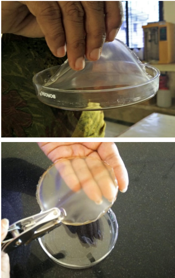
Fig. 3&4 Preparation of alginate films using petri plates
