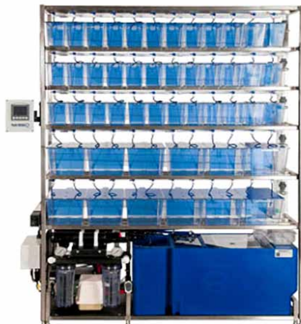
Fig. 3. The recirculating water system for raising laboratory zebrafish
