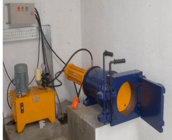
Figure 6: Electrically operated compactor used for solid radioisotope materials compaction process with aluminium containers (1/4) prior to the disposal into dedicated pits.
