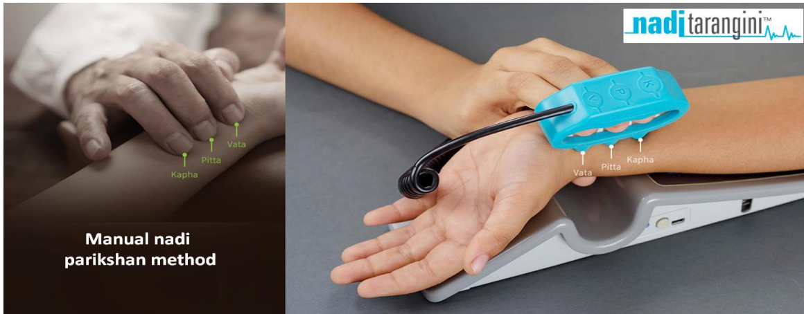
Figure 2. Manual nadi pariksha is done at VPK locations on the wrist using index, middle and ring fingers respectively. Nadi Tarangini mimics the methodology using three pressure sensors which are used at the three locations to record nadi data in real time.
