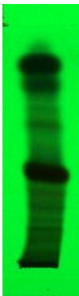
Figure No 11: TLC plate view of bhavitha choorna of dried rhizome of Curcuma longa Linn. at 254nm wavelength
