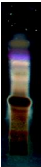
Figure 13: TLC views of methanol extract of bhavitha choorna of dried rhizome of Curcuma longa Linn. after derivatization at 366nm.
