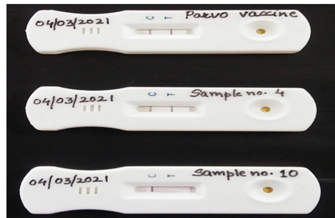
Fig. 1: Antigen Based Lateral Flow Assay for the detection of Canine Parvovirus-2 (CPV-2) from faecal samples from clinical dog samples. A. Parvovirus vaccine (Positive control):- Positive; Sample no.4 :- Positive; Sample no.10 :- Negative
