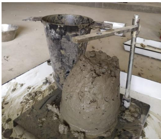
Figure 3: Slump test for fresh concrete
