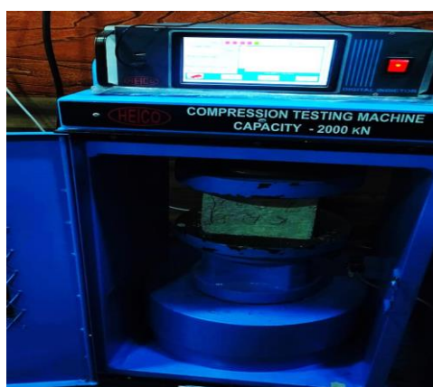
Figure 4: Compressive strength test
