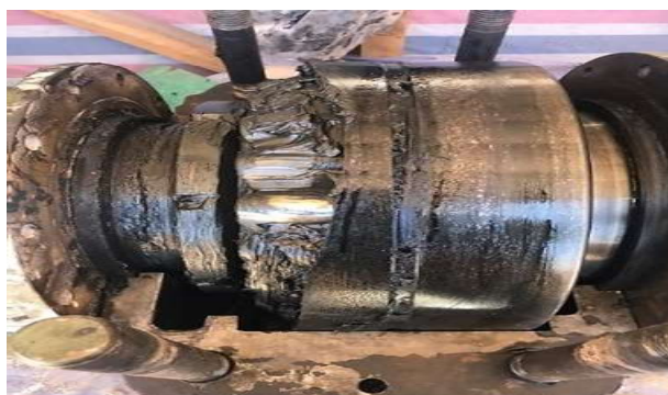
Figure 5: Pinion bearing crack failure outer race
