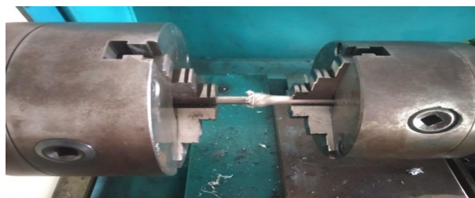
Figure 4: Setup for trail welding
