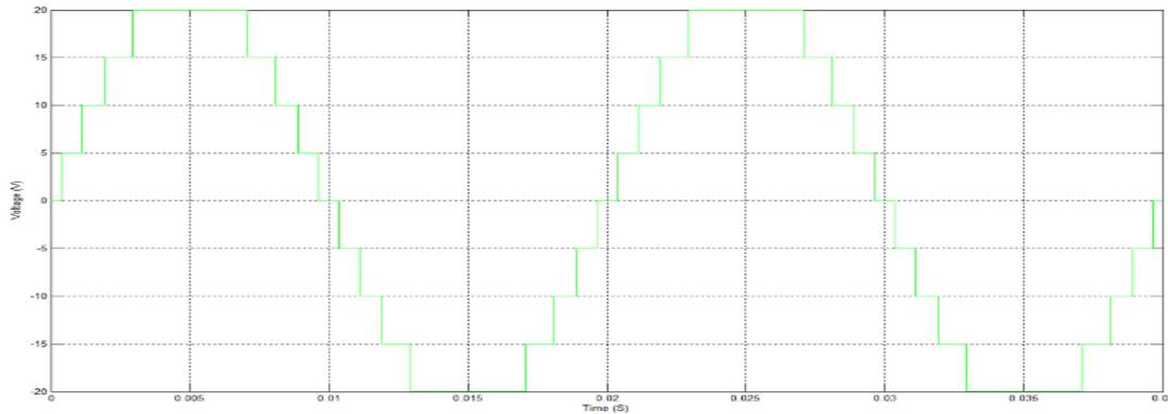
Figure 7: Nine voltage levels in the output waveform of the simulated NLI in 50Hz frequency with R-load
