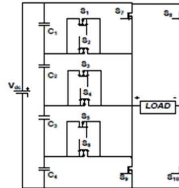
**Figure 1: Proposed topology for nine level inverter (NLI)**
