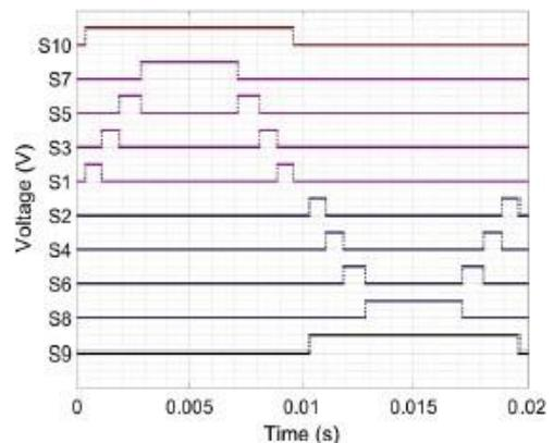
Figure 4: Pulses that turn on the 10 switches
