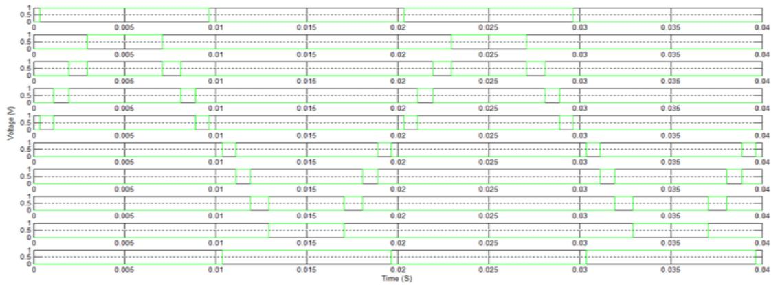
Figure 6: Turning ON pulses for the ten switches
