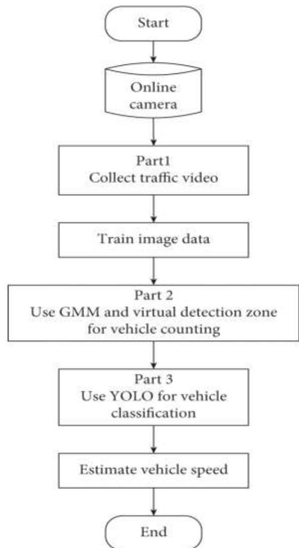
Figure 1 : Flowchart of the vehicle counting and classification process
