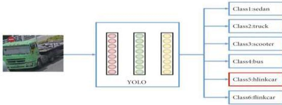
Figure 3: Architecture of visual classifier based on the YOLO algorithm for verifying the vehicle classification.
