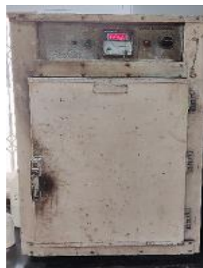
Oven maintaining temp at 100°C
