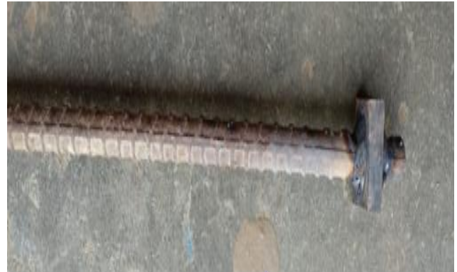
Figure 2: The headed bar
