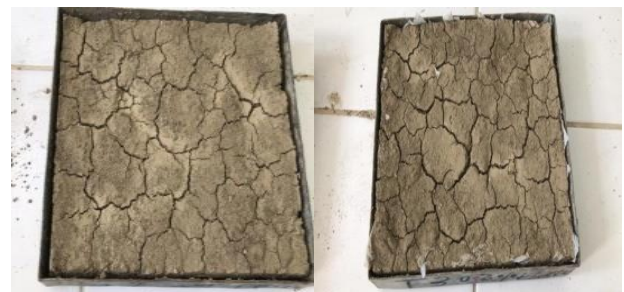
Figure 6: Showing samples with (a)0%, (b)0.2%, (c)0.3% and (d)0.4% after drying/shrinkage.
