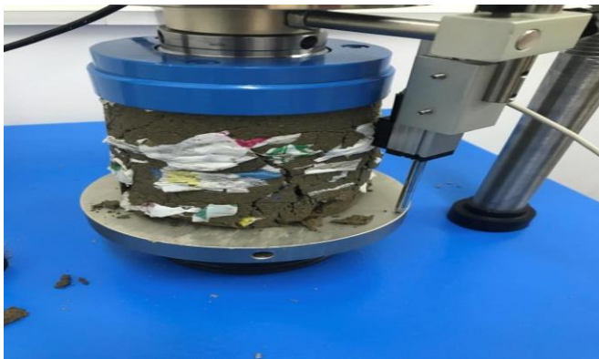
Figure 5: UCS result showing the failure under stress for 0.4% plastic content
