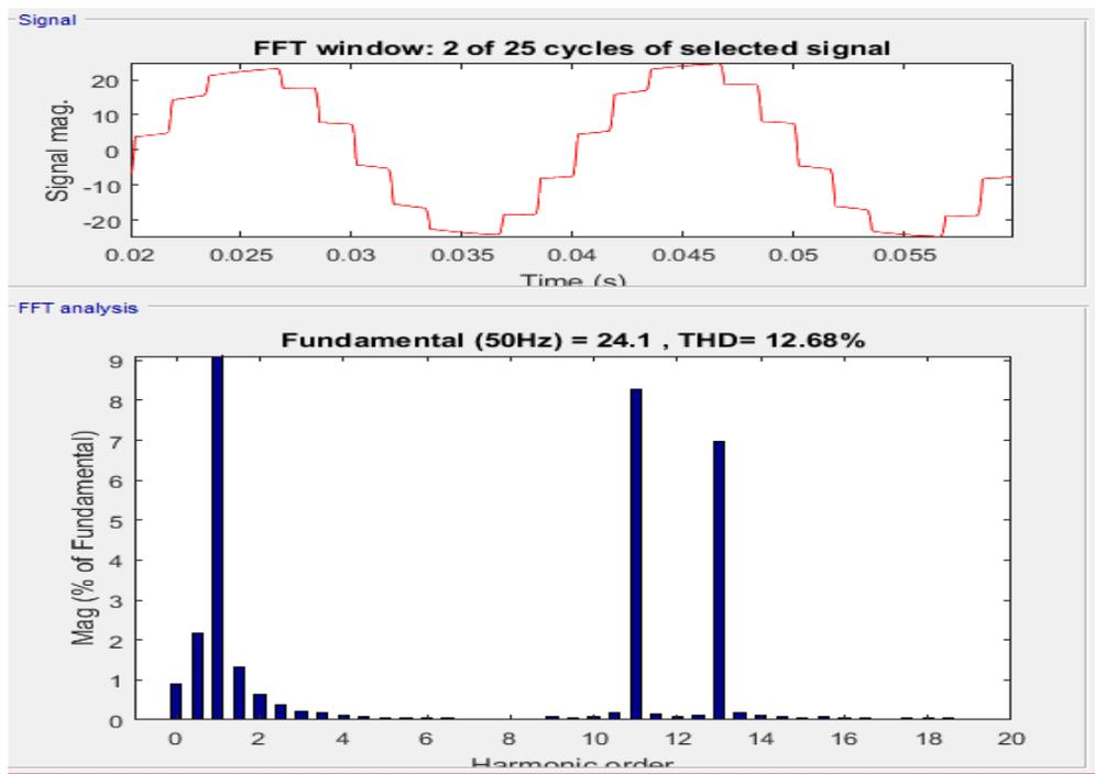
Figure 8: FFT analysis of grid side current (isa) of 12 pulse rectifier
