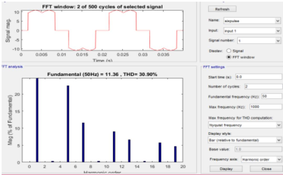
Figure 5: FFT Analysis of 6 pulse rectifier
