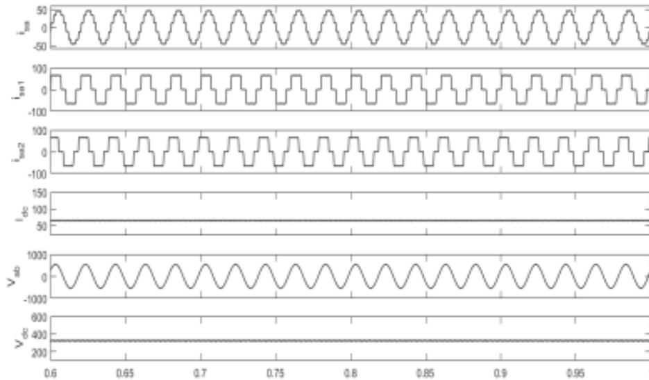
Figure 7: Results of 12 pulse rectifier
