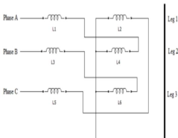
Figure 1: Zig-Zag Coupling for Positive Phase Shift
