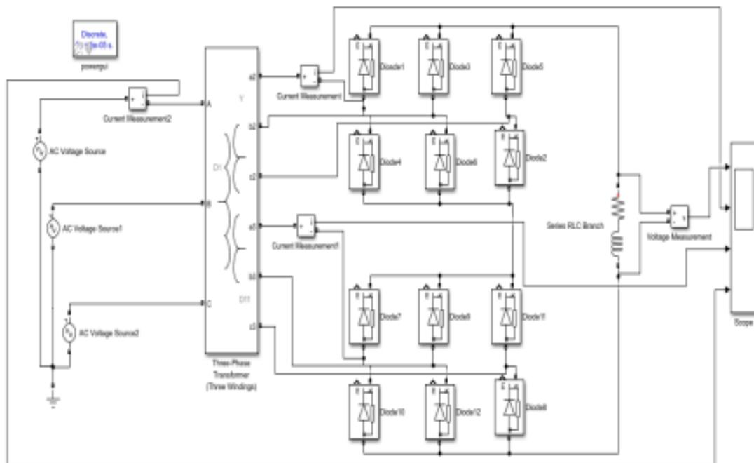
Figure 6: Simulation diagram of 12 pulse rectifier
