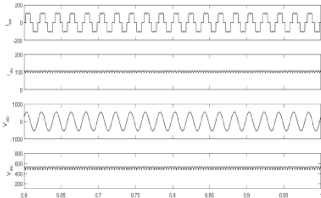
Figure 4: Results of 6-pulse rectifier
