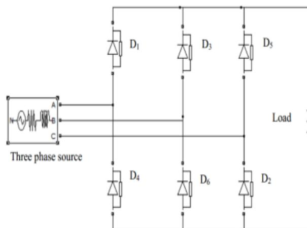
Figure 2: Circuit Diagram of a Three Phase Rectifier
