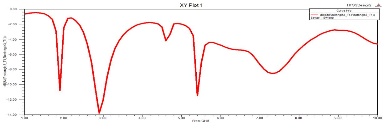
Figure 2: Simulated Reflection Coefficients of Antenna Iterations
