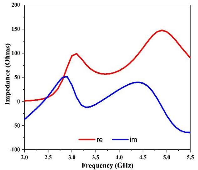
Figure 6: Impedance characteristics of the proposed antenna
