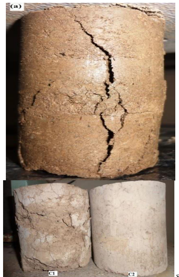
Figure1: Failed Specimen in UCS
