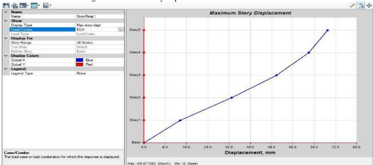
Figure 6: Maximum story displacement without retrofitted column
