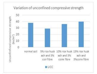
Figure 4: Variation of Unconfined Compressive Strength
