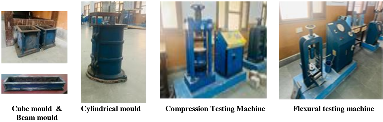
Figure 3: Equipments/moulds used for preparing and testing of concrete
