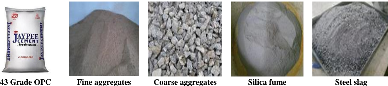
Figure 1: Materials used Cement, Sand, Aggregates, Silic Fume & Steel Slag
