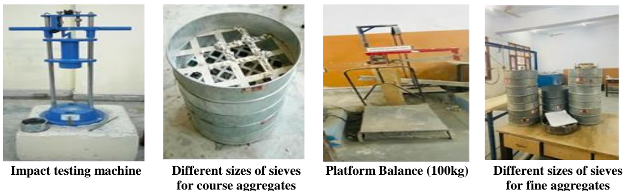
Figure 2; Various equipments used for material testing
