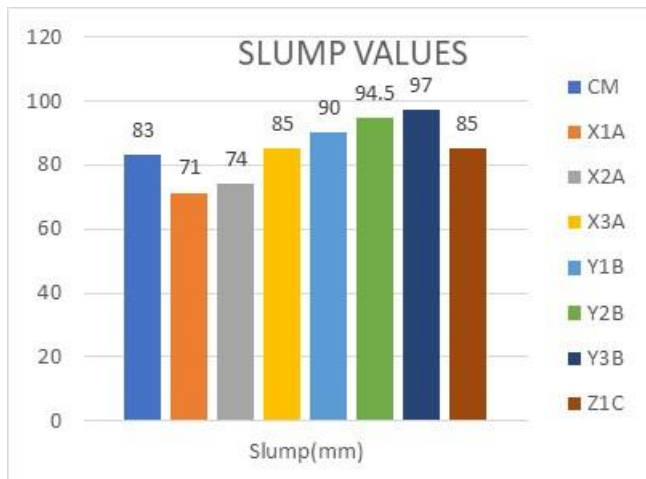
Figure 9: Effect on workability (Slump test)
