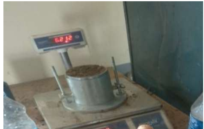
Figure 1: California Bearing Ratio Test
