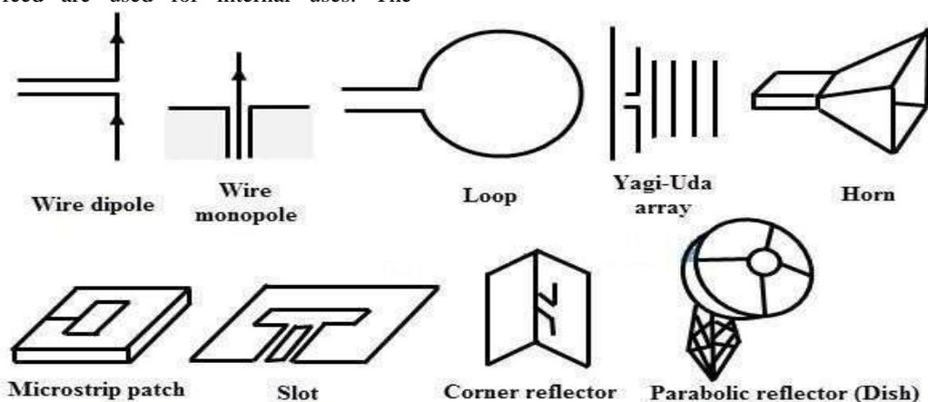
Figure 1: Block diagram basic antenna structure
