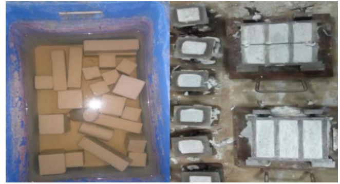
Figure 8: Casting and Curing
