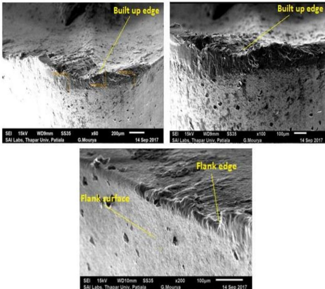
Figure 8: K10 tool SEM micrographs (a) 60X (b) 100X (c) Flank surface 200X
