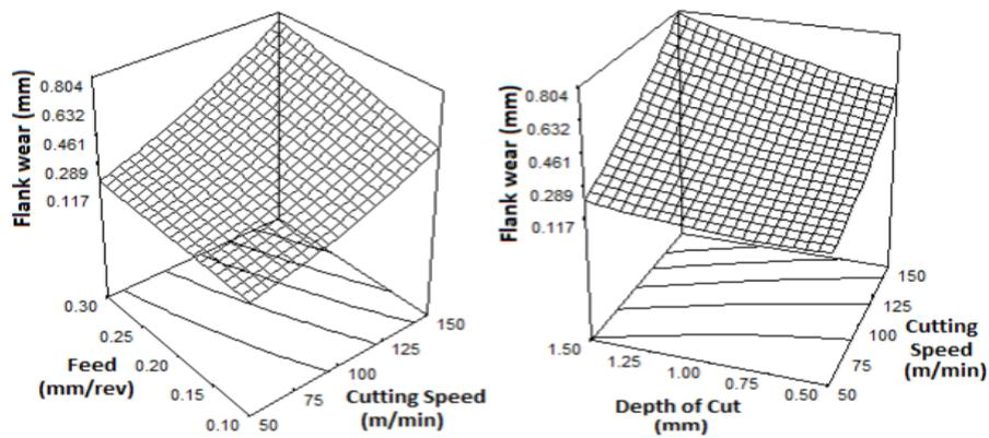
Figure 7: Flank wear response surfaces
