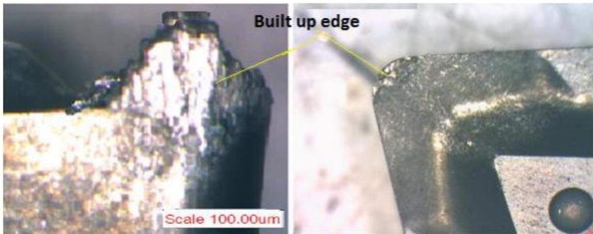
Figure 6: BUE image at S=50m/min, F=0.2mm/rev, and D=1.5mm
