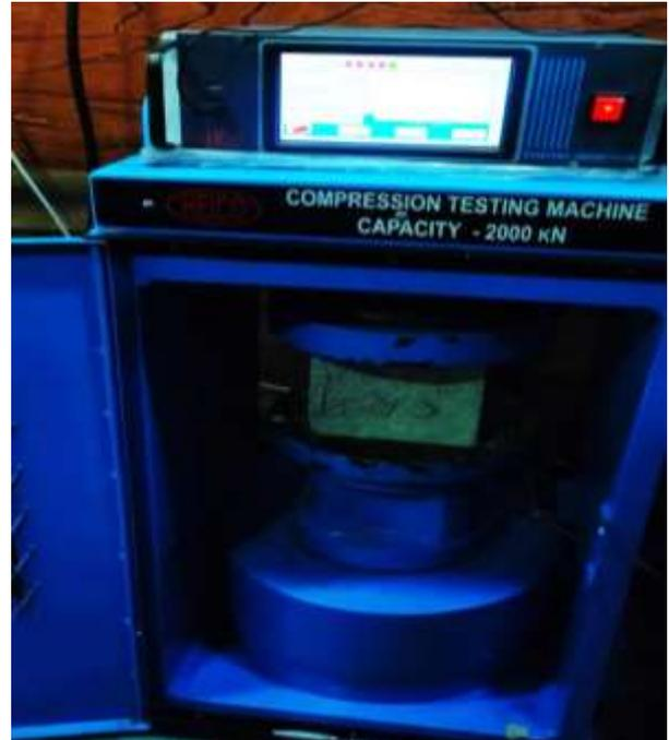
Figure 4: Compressive strength test
