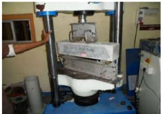
Figure 5: Flexural strength test
