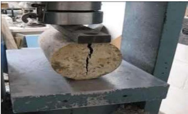
Figure 6: Split tensile test
