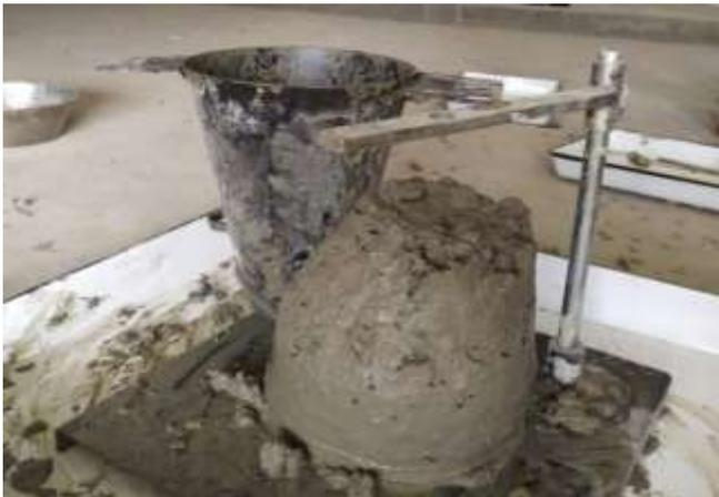
Figure 3: Slump test for fresh concrete
