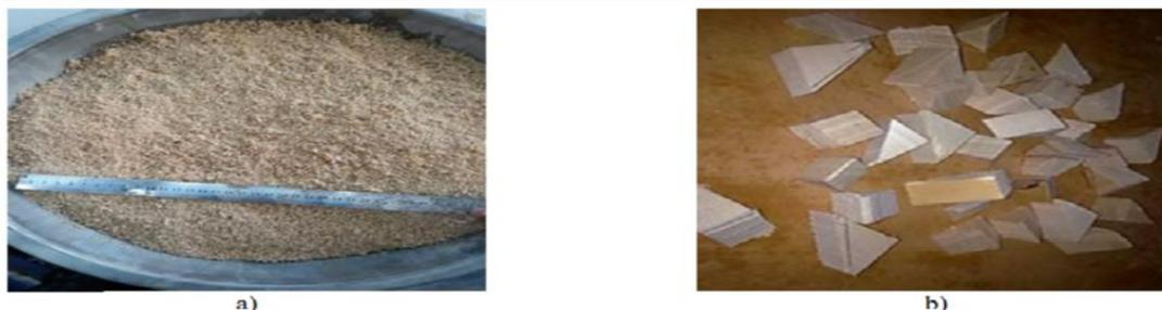
Figure 2: Wood waste: a) Sawdust Waste (SW), b) Wood Waste Aggregate (WWA) (Abed et al. 2019).
