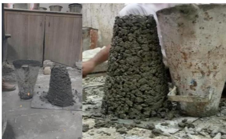
Figure 4: Conducted a slump test (Soomro et al. 2021)
