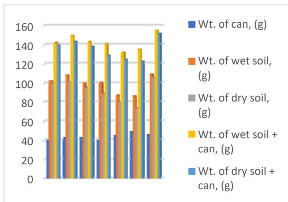
Figure 15: Standard Proctor Compaction Investigation
