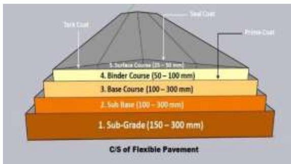
Figure 2: Flexible Pavement
