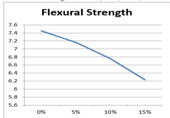
Figure 4: Flexural Strength for 0%, 5%, 10%, 15% replacement of Fine Aggregate by Crumb Rubber
