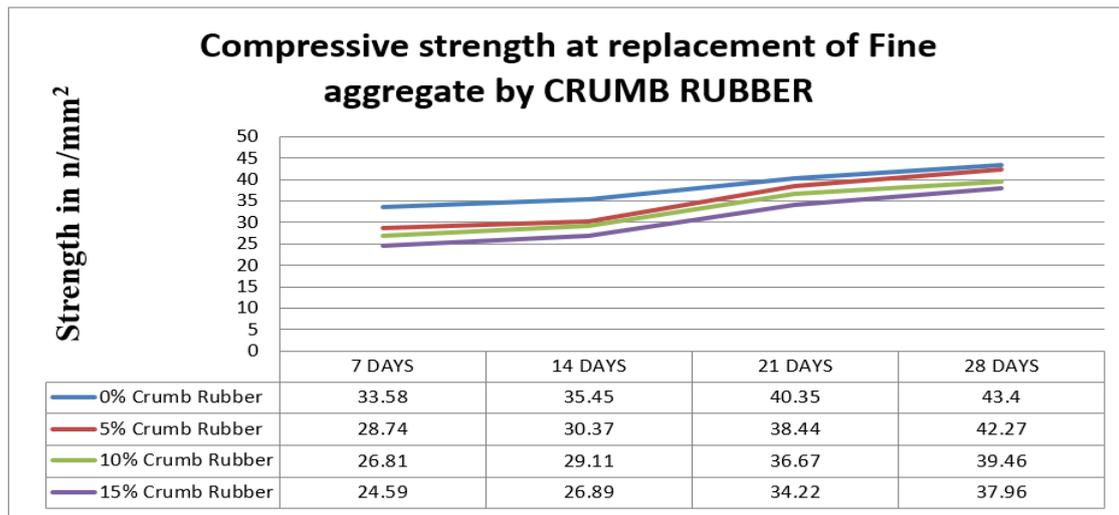
Figure 6: Compressive strength at 0%, 5%, 10% & 15% replacement of Fine Aggregate by Crumb Rubber after 7,14,21 & 28 days (M-35)
