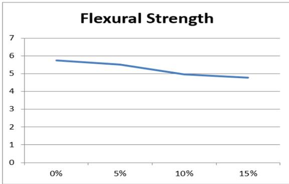
Figure 3: Flexural Strength for 28 days varying from 0%, 5%, 10%, 15% replacement of Fine Aggregate by Crumb Rubber
