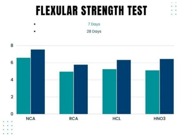
table no: 5.3. Flexural strength test results after 7days and 28 days.
