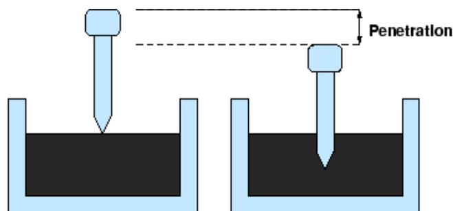
Figure 1: Penetration test setup
