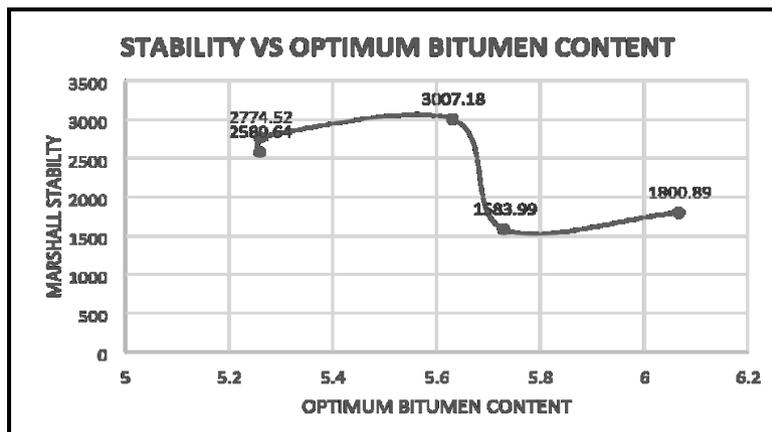
Figure 3: Comparative result between Stability VS Optimum Bitumen Content
