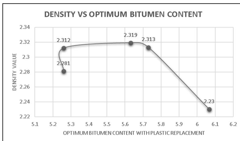
Figure 4: Comparative result between Density VS Optimum Bitumen Content
