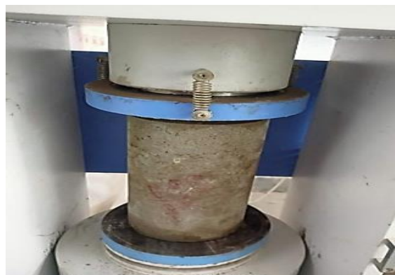
Figure 3: Compressive Strength Test Specimen
