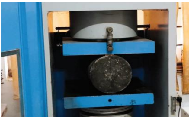
Figure 8: Split Tensile Strength Test Setup
