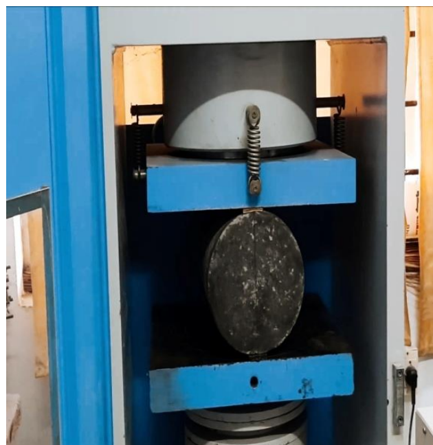
Figure 5: Split tensile strength test setup
