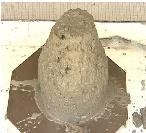
Figure 3: Slump test for fresh concrete
