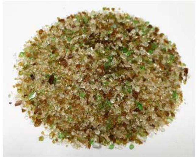
Figure 1: Crushed waste glass particles
