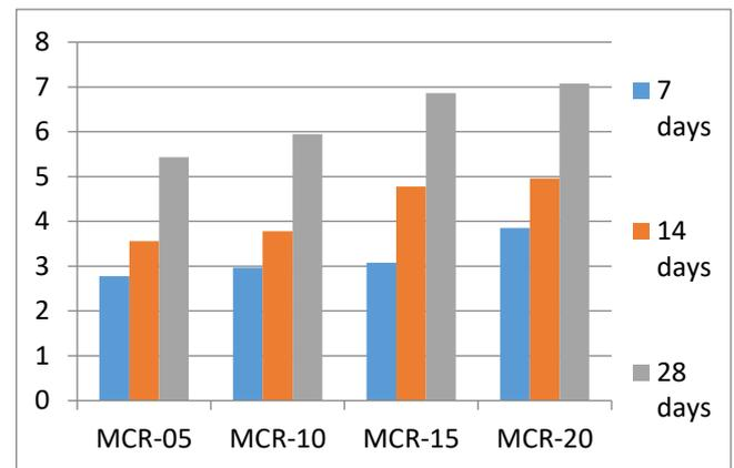
Figure 3: Graph showing the flexural strength of cubes in 7,14 and 28 days
