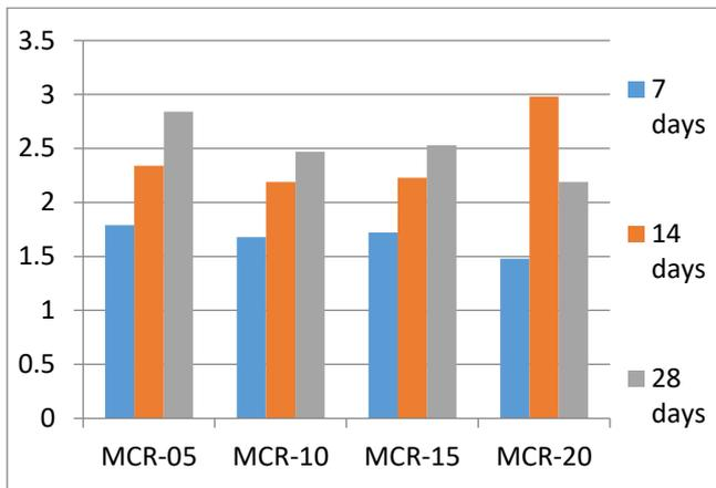
Figure 4: Split tensile strength of cylinders in 7, 14 and 28 days
