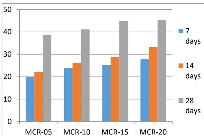
Figure 2: Compressive strength of cubes in 7,14 and 28 days
