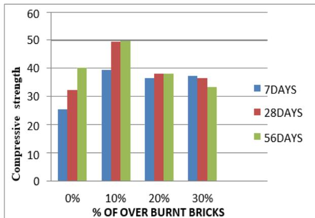
Figure 3: Variation of Compressive Strength gives the higher strength for the replacement 10% for 7, 28 and 56 days by over burnt bricks
