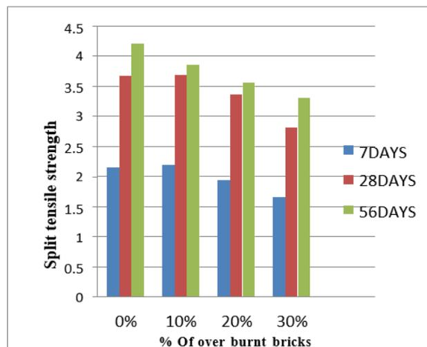
Figure 5: Variation of Split tensile Strength gives the higher strength for the replacement 10% for 7, 28, 56 days by over burnt bricks
