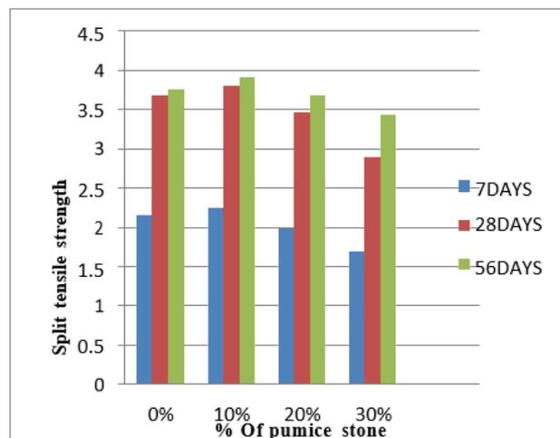
Figure 6: Variation of Split tensile Strength gives the higher strength for the replacement 10% for 7, 28, 56 days by pumice stone
