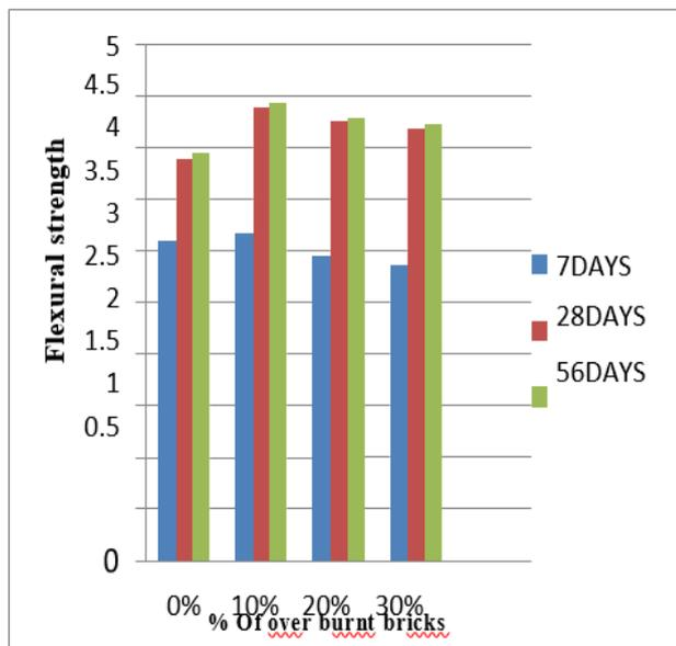
Figure 7: Variation of Flexural Strength gives the higher strength for the replacement 10% for 7, 28, 56 days by over burnt bricks
