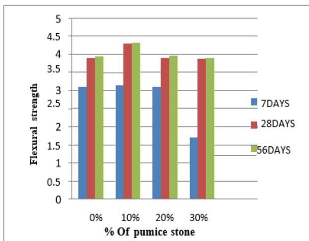
Figure 8: Variation of Flexural Strength gives the higher strength for the replacement 10% for 7, 28, 56 days by pumice stone
