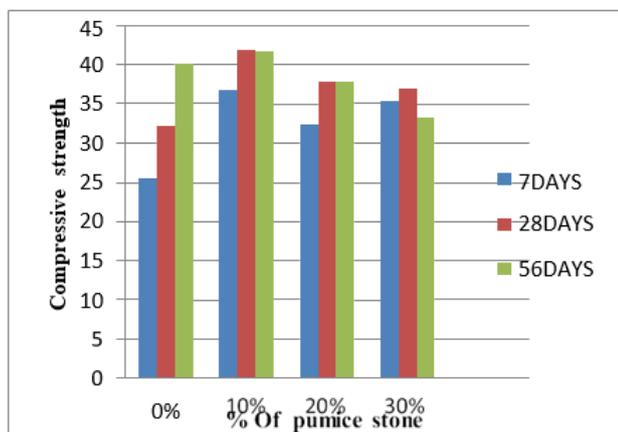
Figure 4: Variation of Compressive Strength gives the higher strength for the replacement 10% for 7, 28 and 56 days by pumice stone
