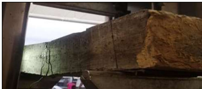
Figure 5: Failure Photo of Beam Bo-1
