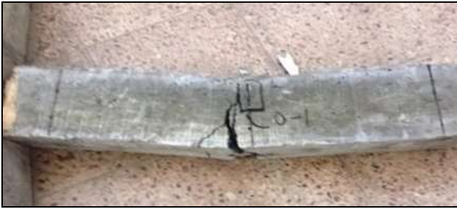
Figure 8: Failure Photo of Beam Co-1
