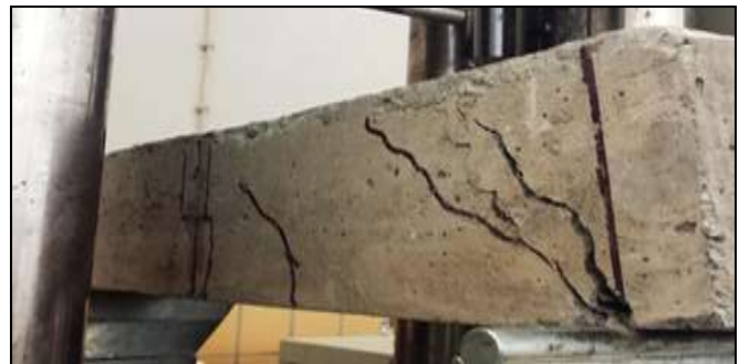
Figure 6: Failure Photo of Beam B-3
