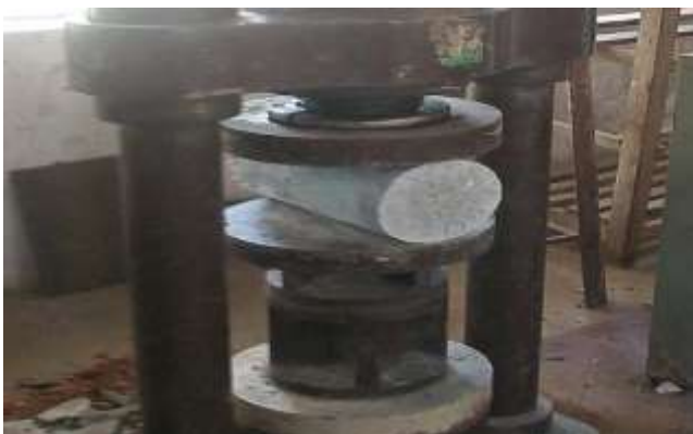
Figure 11: Splitting tensile strength test set-up
