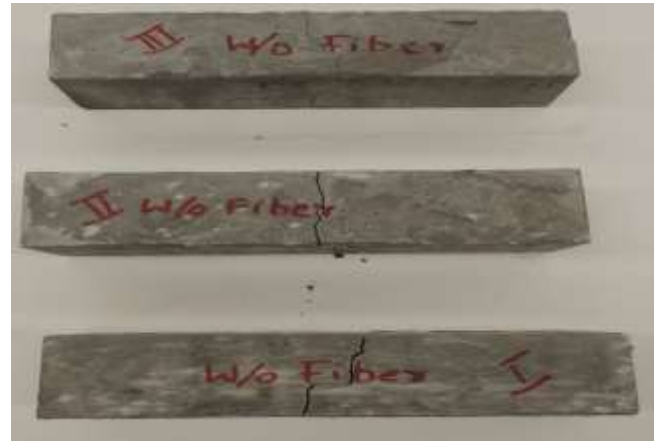
Figure 17: Cracks pattern of PFC concrete specimen I, II and III
