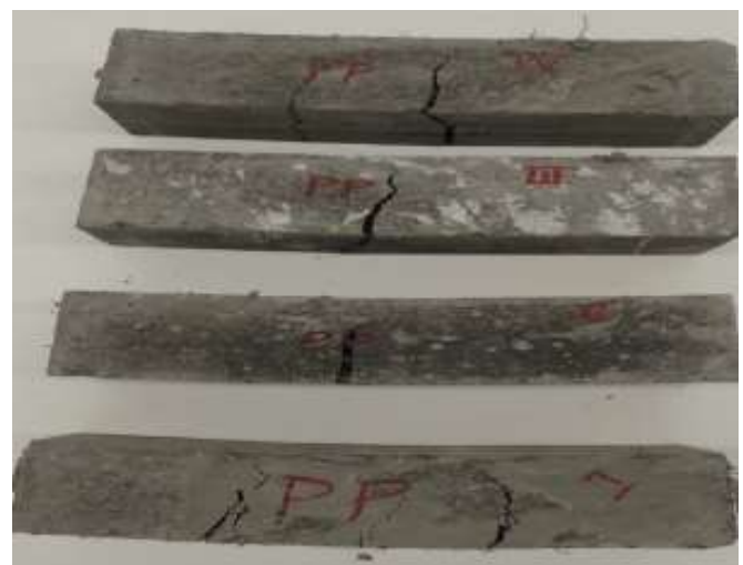
Figure 18: Cracks pattern of PPFC concrete specimen I, II and III.
