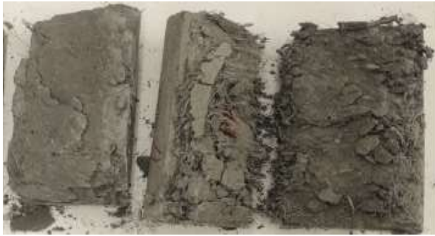
Figure 15: Crack pattern of concrete made with PFC, PPFC and BFC.
