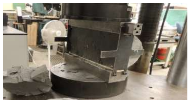
Figure 14: PFC failure pattern of concrete sample
