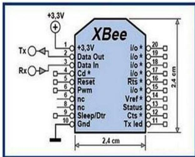
Figure 6 Zigbee pin configuration
