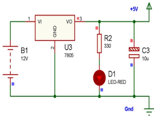
Figure 9 Battery operated +5V power supply
