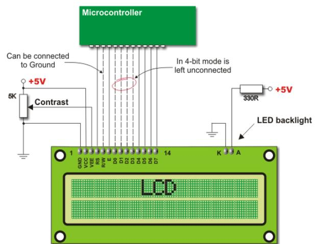
Figure 8 LCD Basic Connection
