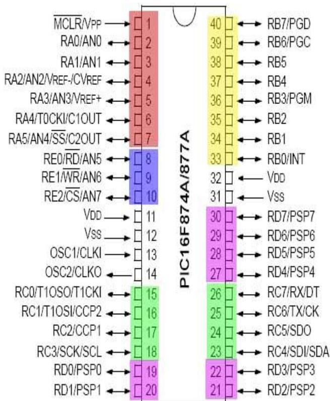
Figure 7 PIC 16F877A Pin Configuration
