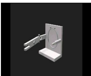
Fig.36 Fixture in open clamp position
