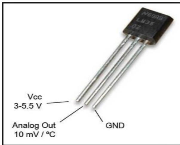
Fig. 6: Temperature Sensor
