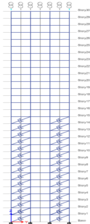
Fig 10: Viscous Damper up to 15 th floor.
