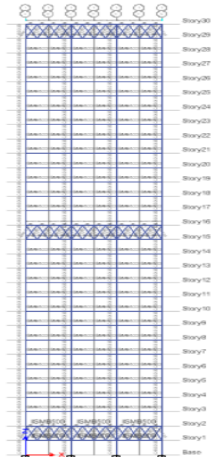
Fig. 6: Truss Belt System Elevation View
