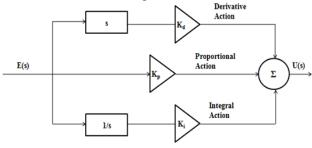
Fig. 1: PID Controller
