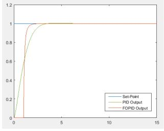
Fig. 5: Comparison of Conventional PID controller with FOPID controller
