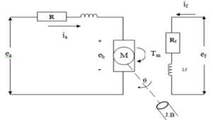
Fig. 3: Separately Excited DC Motor with constant Field Current
