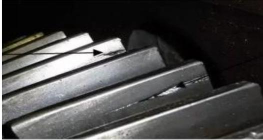
Fig 3: Teeth cracks near gear root due to low bending stress of material
