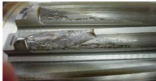
Fig 1: Spalling of helical gear teeth
