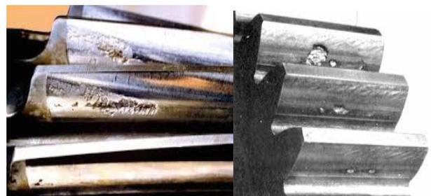
Fig 2: Crates and Pores due to pitting corrosion in spur gears
