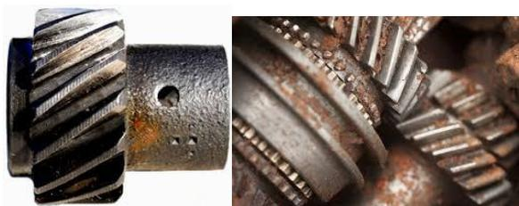
Fig 5: Brown coloration of materials due to corrosion
