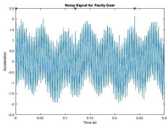
Fig 8: Noisy Signal for Faulty Gear
