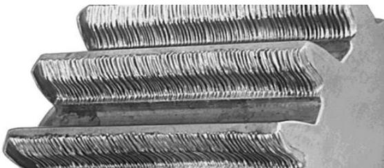
Fig 4: Fine lines over material due to abrasive particles
