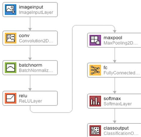
Fig 9: Block diagram showing the designed network layers
