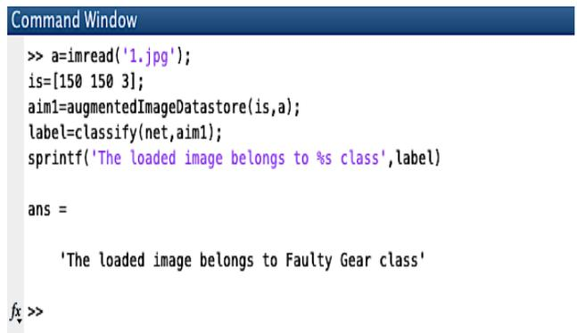
Fig 12: Output of trained model showing results of gear class
