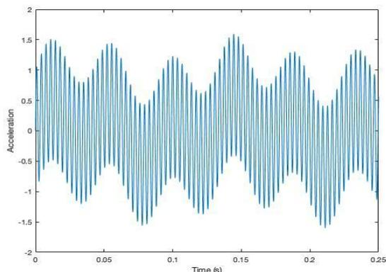
Fig 6: Gear mesh signal analysis for healthy gears of a gearbox
