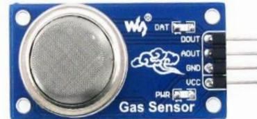
Fig. 5: MQ-7 Gas Sensor
