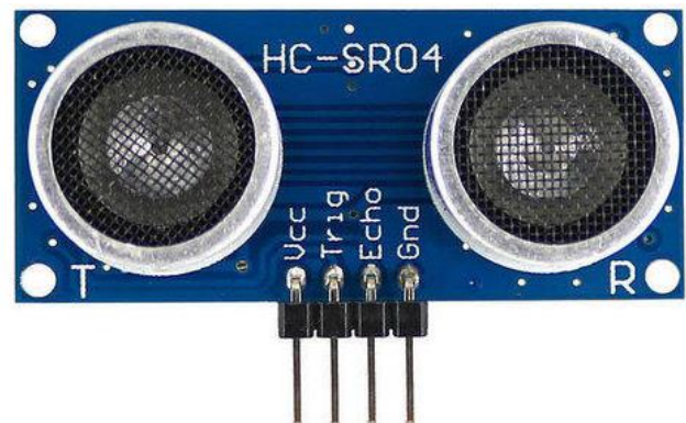
Figure 3: Diagrammatic Representation of ultrasonic sensor [ELECTRONIC HUB]
