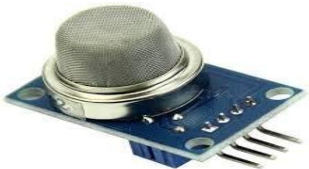
Figure 5: Illustrates the module of smoke sensor use for detecting smoke[22]
