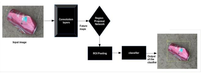
Figure 3: System Architecture Based on Faster RCNN
