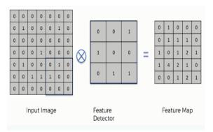
Figure 4: Illustrating the Convolution operation
