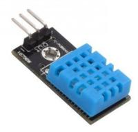
Figure 5: The above diagram shows the module of Temperature sensor [9]
